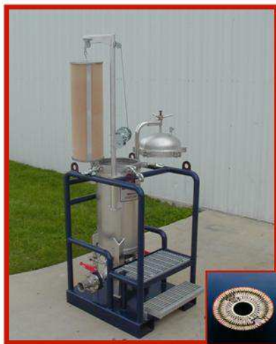
Figure 8 / HCCF filter and housing
