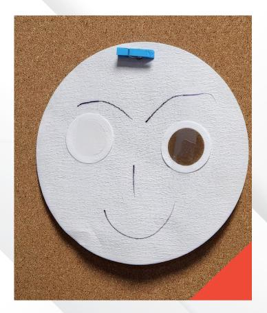
Process clarified that the circle on the right is the finished product from the 1 micron absolute bag. This cleanliness level barely passes. On the left is one pass through the 0.5 micron glass. It passes easily. This example is hanging in the plant managers office.
