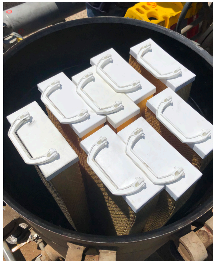
Eight Invicta™ cartridges after installation in the customer's upgraded vessel
