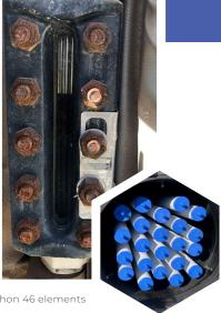
Before (left) and after (right) Cyphon 46 elements were in service for 60 hours.
