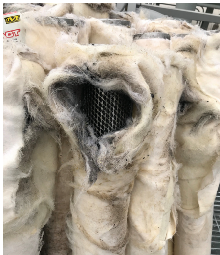
Figure 3 Damaged Coalescing Elements Demonstrating Bypass
