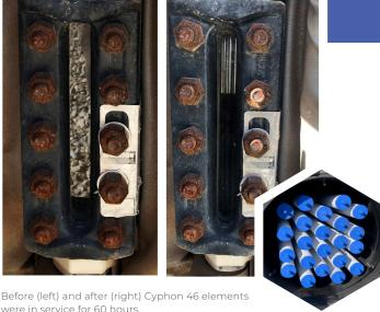
Measurable liquids were almost immediately seen in the first and second stage sight glasses after the Cyphon 46 elements were installed.
